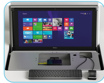
Keyboard tray with detail of Raspberry Pi mounting
