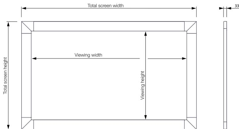
Total frame width = Viewing width + 100mm
