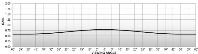
GAIN 0.8 VIEWING ANGLE 180° THICKNESS 0.37 MM FULL HD COMPLIANT
