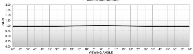
GAIN I.0 VIEWING ANGLE 180° THICKNESS 0.5 MM FULL HD COMPLIANT
