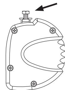
**EN:** Mount the screen on the brackets and tighten the screws (5Nm)
