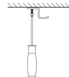
**EN:** Place the nuts together with the screws in the track
