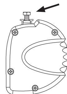
**EN:** Mount the screen on the brackets and tighten the screws (5Nm)
